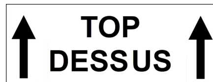
FIGURE 36: TOP ORIENTATION OF I-BEAM
